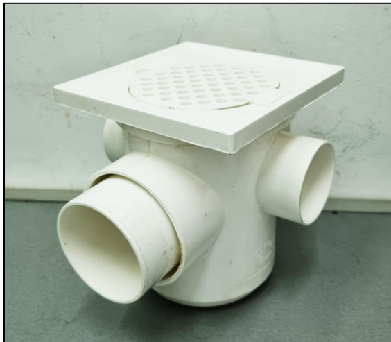
Photo 1 – Gully with grating for flow rate test
